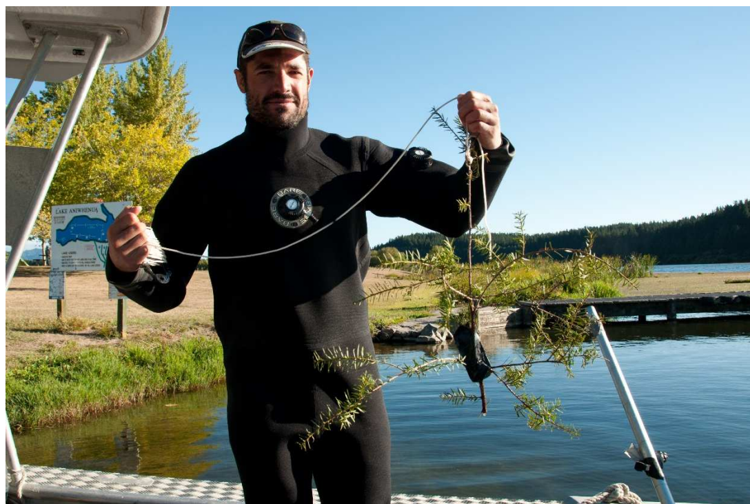
Figure 8: A simple surrogate was used to estimate detection distances in a range of lake water clarities, and compared with Secchi disc depths.
