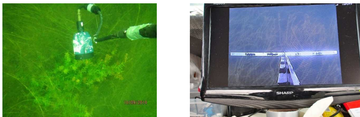
Figure 7: A drop camera deployed for underwater video imagery, and screen viewed results showing a graduated 'T-bar' on the screen deployed to measure field of view.
