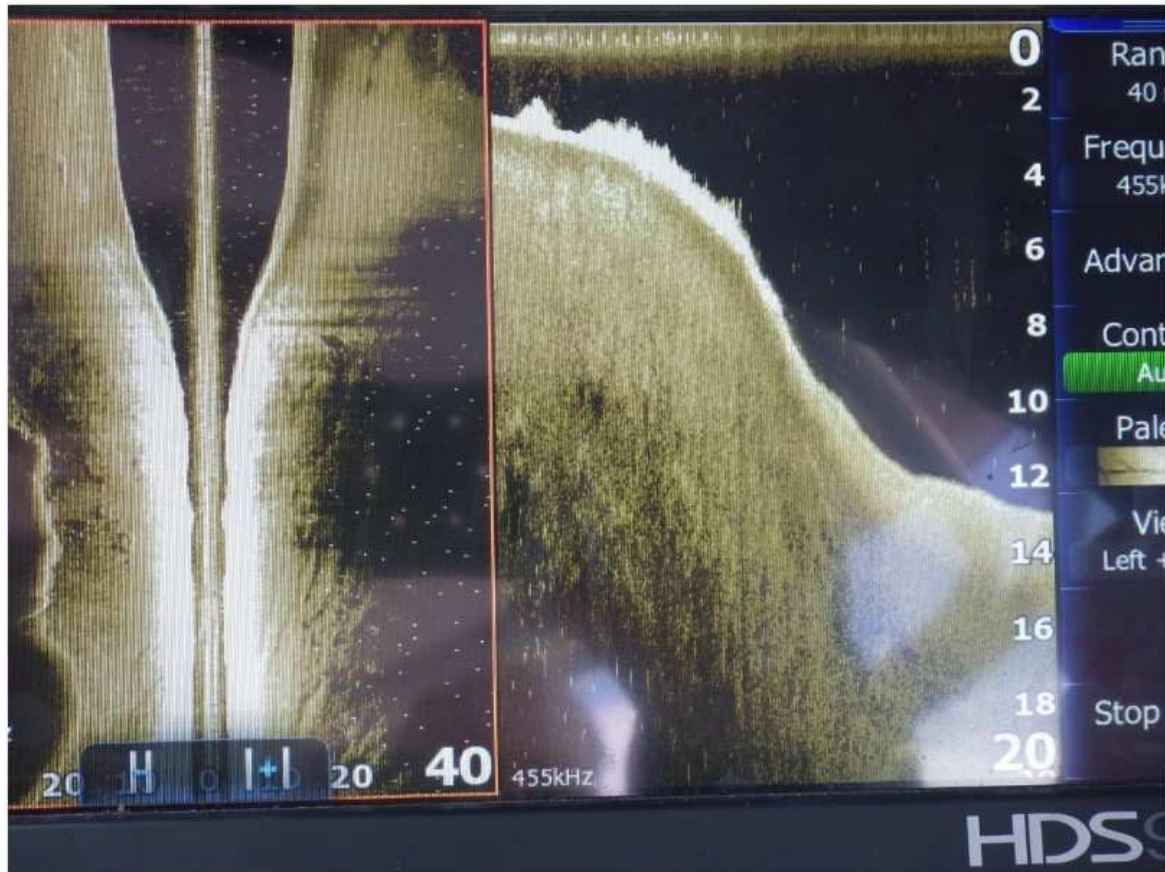
Figure 6: Images of a Lowrance unit and examples of down-scan (top right & bottom right) and side scan (bottom left) output.
