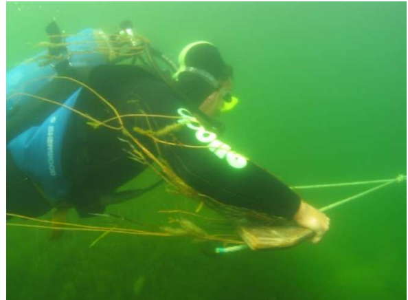
Figure 4: Manta board use gives a diver some manoeuvrability while covering areas at a greater speed than scuba alone.
