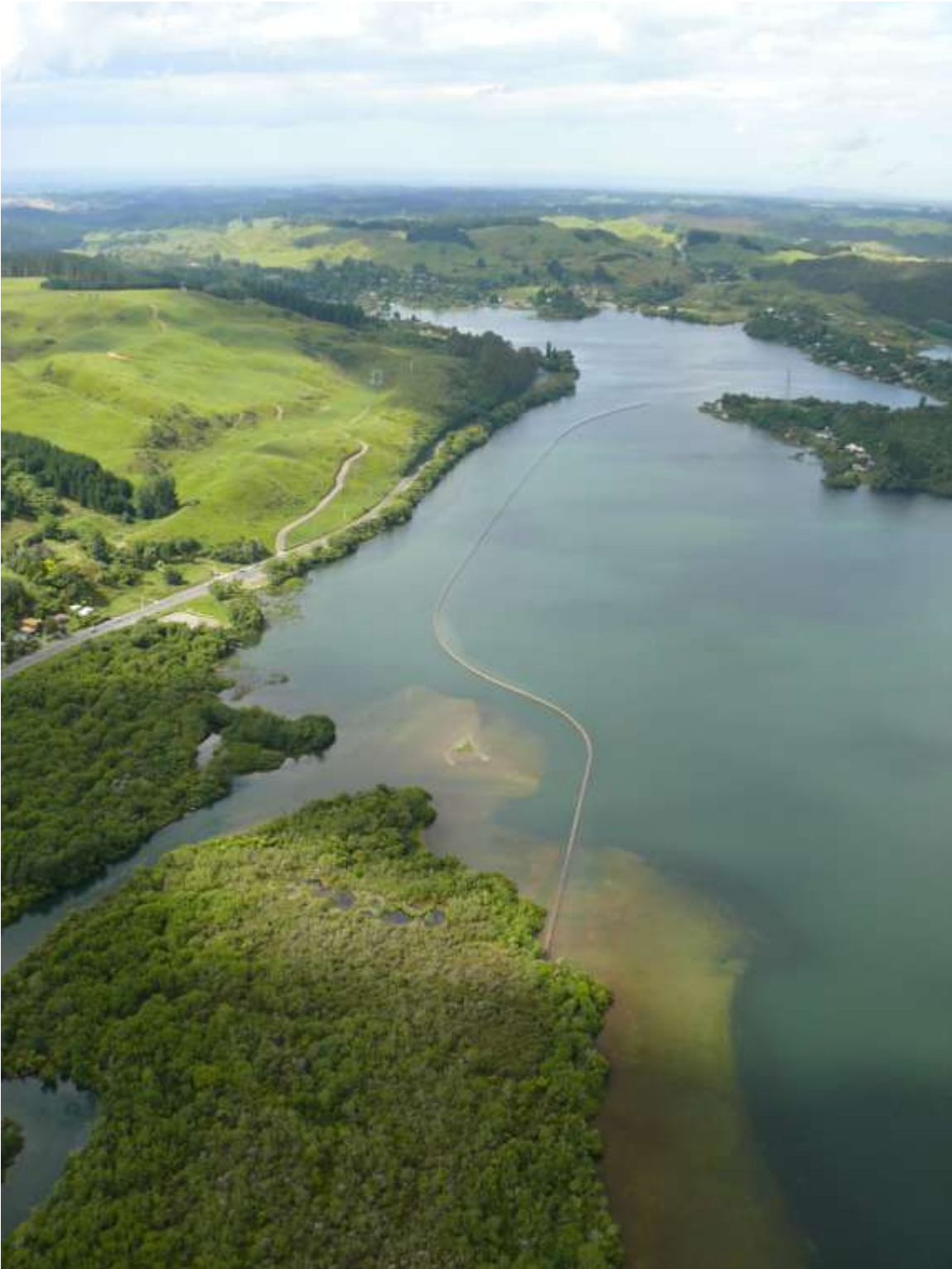
Figure 10. Photo of the Ohau Channel diversion wall showing the Okere Arm towards the outlet of Lake Rotoiti (upper left). Photo: Environment Bay of Plenty.
