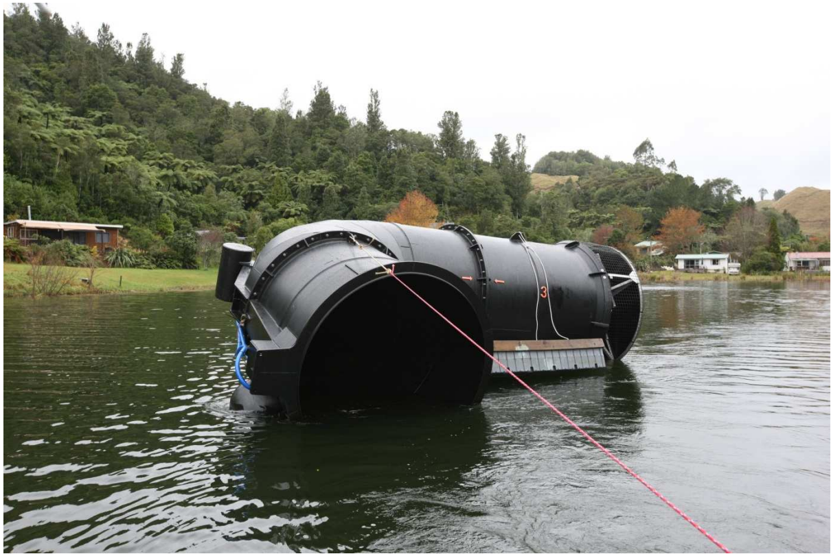
Figure 1: Part of a de-stratification machine being towed into the lake.
