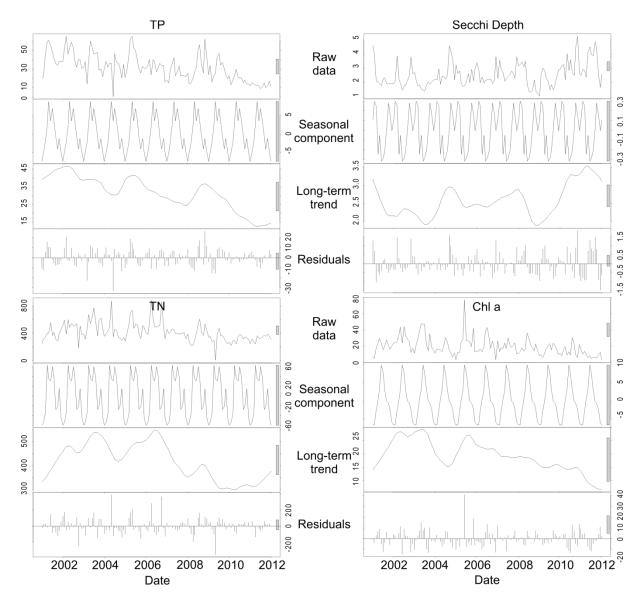
Figure 4.2 Decomposed time-series components for site 5 amongst TLI parameters for the period 17/10/2001-17/10/2012 (units: TP, chl *a* and TN = mg/m<sup>-3</sup>; Secchi depth = m). Daily observations of surface water quality (0-6 m depth) are plotted as the uppermost graph of each TLI parameter, followed by the seasonal component (12-month period), long-term trend (loess smoothed) and residuals in corresponding units
