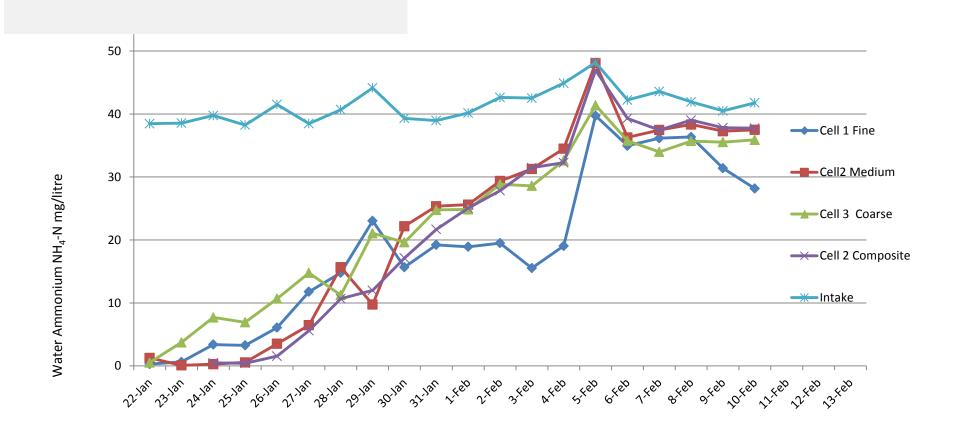
Part 1, three grades of zeolite - Coarse, Medium and Fine using 150 litres/hr per cell flow rate which is 50% of previous (phase 1) flow rate. Cells operate in parrellel.
