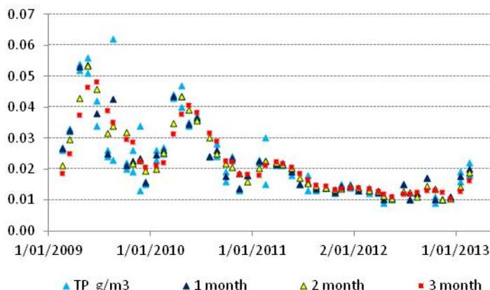
Figure 2 The total phosphorus (g/m<sup>3</sup>) data from two sites in Lake Rotorua with the one monthly, two monthly and three monthly averages.
