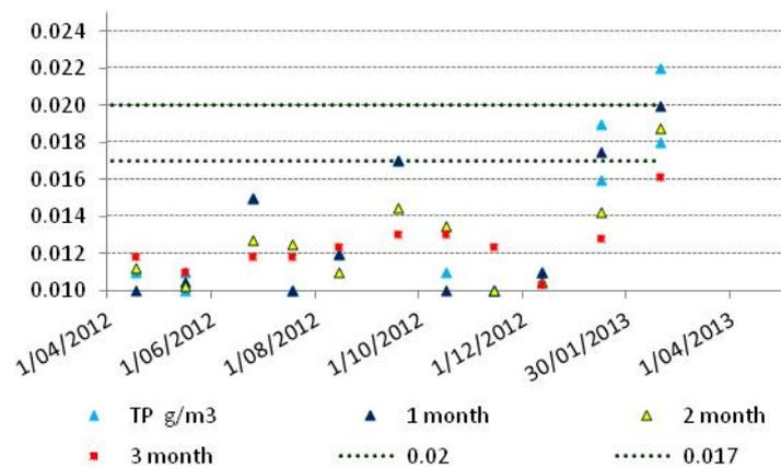
**Figure 3** The total phosphorus (TP) concentration in Lake Rotorua from 2 sites, with the one, two and three monthly average TP concentrations and the control band between 0.017 and 0.020 g/m<sup>3</sup> TP, from monthly sampling between April 2012 and February 2013.
