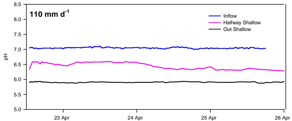
**Figure 23:** pH within the low loaded chamber (April 2010).
