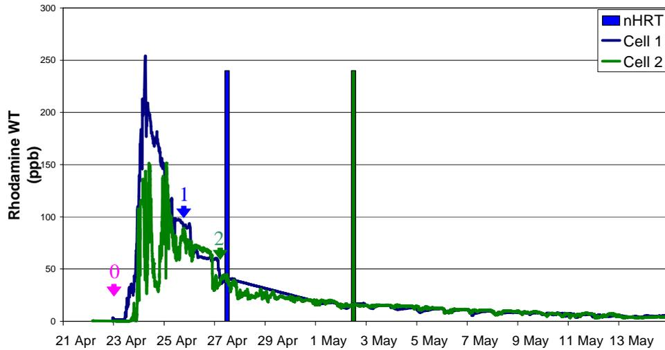
**Figure 27:** Rhodamine WT tracer from both cells of the high loaded chamber. Arrows indicate: time of tracer addition (0), tracer centroid for cell 1 (1) and cell 2 (2). The Nominal (or theoretical) retention times for each cell are shown as bars.
