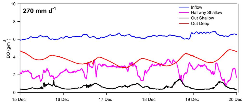
**Figure 16:** Dissolved oxygen concentrations measured within the high loaded chamber (Dec 2009).
