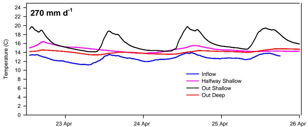
**Figure 14:** Temperatures measured at various locations within the high loaded chamber during April 2010.
