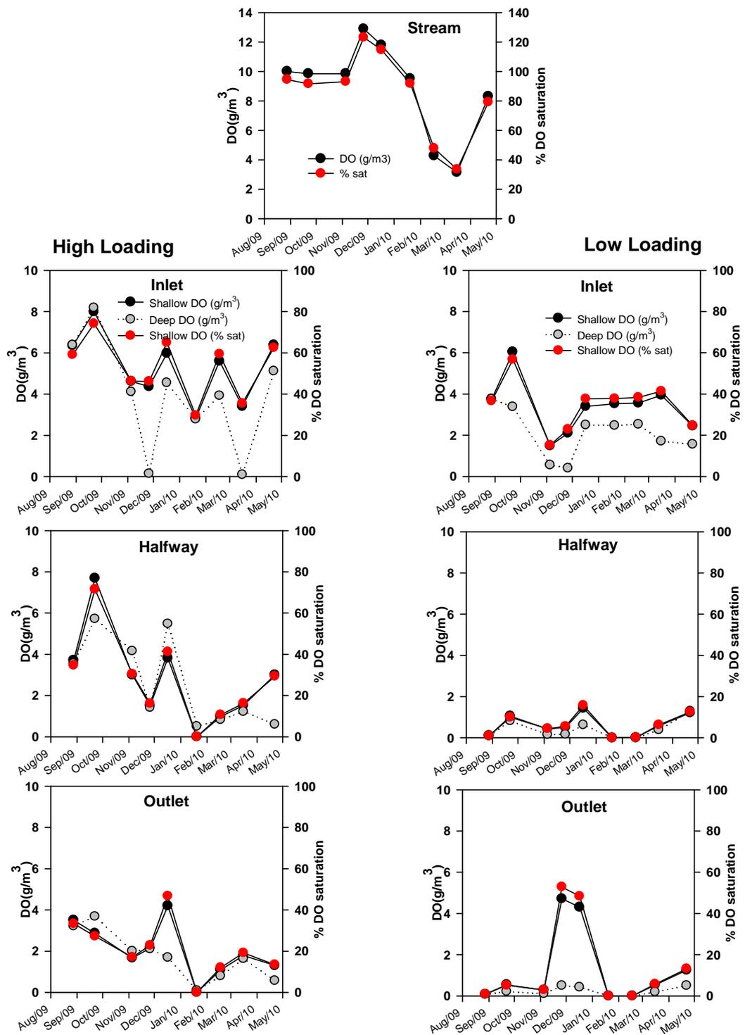
**Figure 14:** Dissolved oxygen data for stream (top), chamber water column at inlet, halfway and outlet positions (shallow and deep) for high loaded chamber (left) and low loaded chamber (right).
