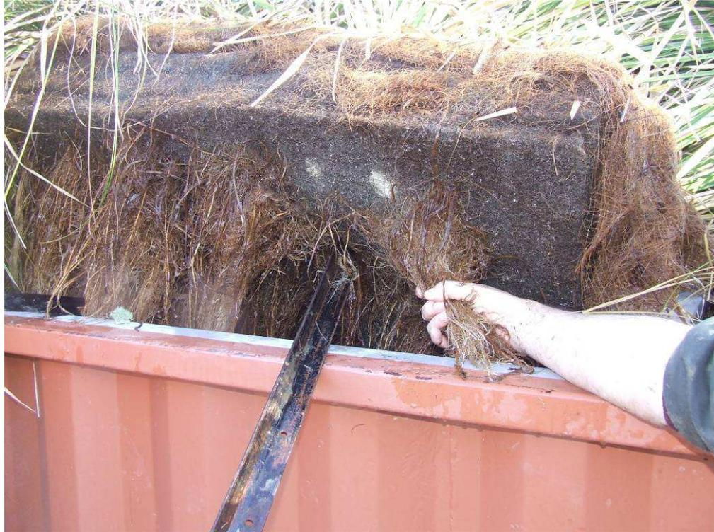
**Figure 10:** Section of FTW where root development was sufficiently restricted to demonstrate that the harvested area along one edge approximated the width of roots from the outer row of plants.
