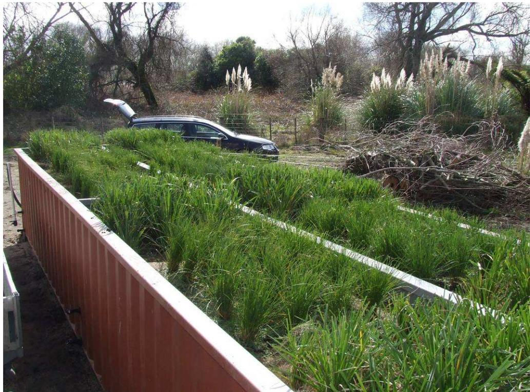
**Figure 5:** Mesocosm tanks with FTWs installed.
