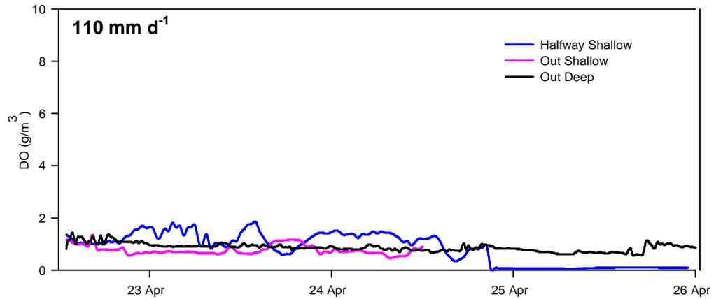
**Figure 19:** Dissolved oxygen concentrations measured within the low loaded chamber (April 2010).
