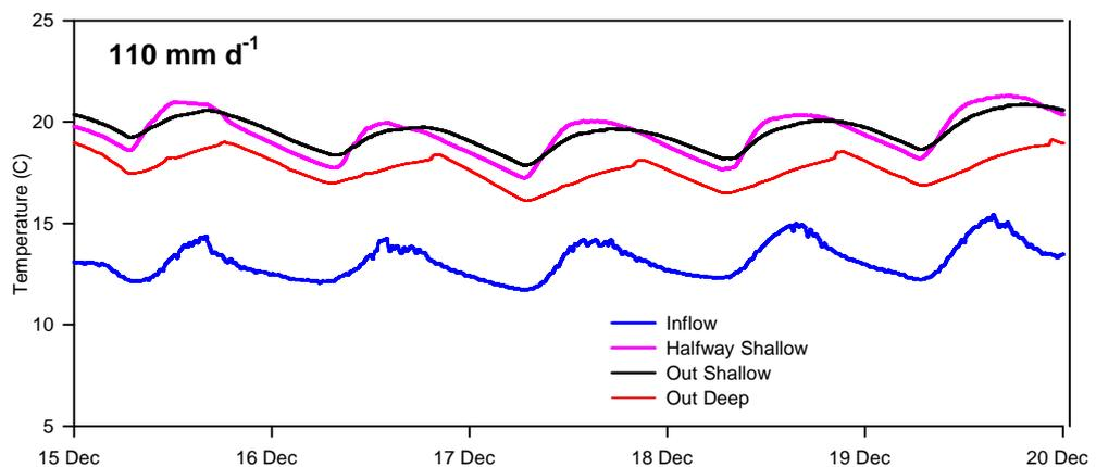
**Figure 13:** Temperatures measured in the low loaded chamber (Dec 2009).
