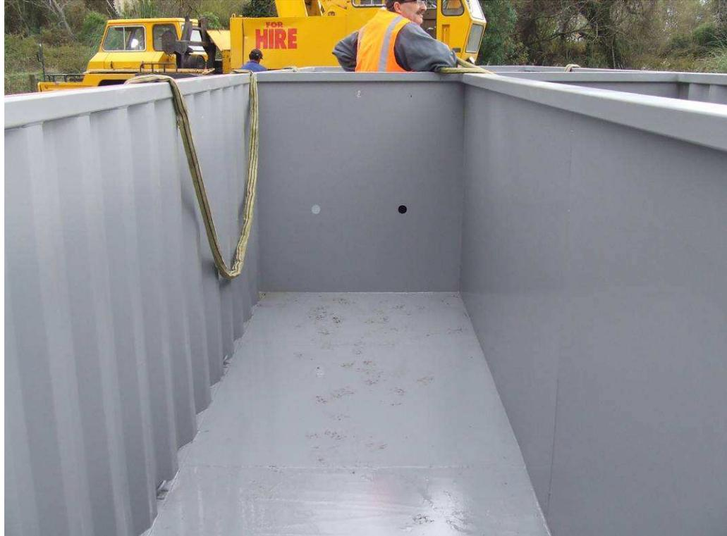
**Figure 3:** Internal view of an empty mesocosm tank, showing central wall dividing each chamber into two cells. The two holes through which water flows are also visible.
