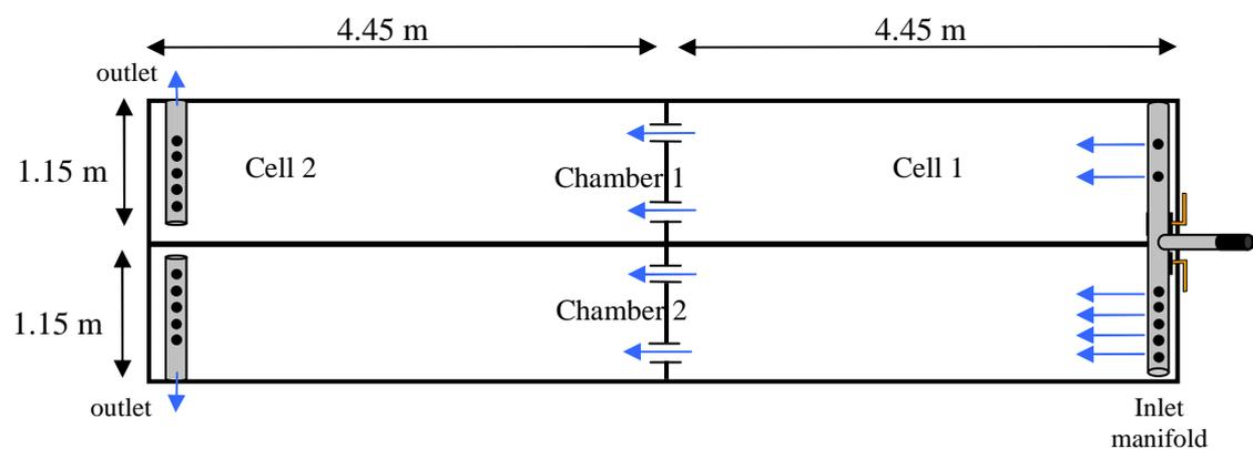
**Figure 2:** Plan view of the mesocosm tanks. The inflow enters on the right and exits on the left side of the diagram.
