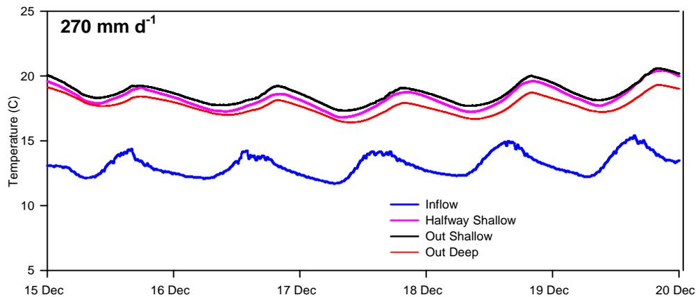
**Figure 14:** Temperatures measured in the high loaded chamber (Dec 2009).
