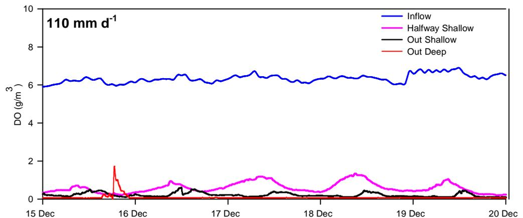
**Figure 17:** Dissolved oxygen concentrations measured within the low loaded chamber (Dec 2009).
