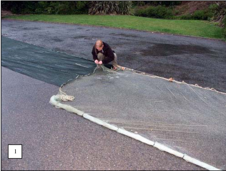
Plate 1. Enclosure net, showing the main net and the synthetic garden shade cloth end attachments.
