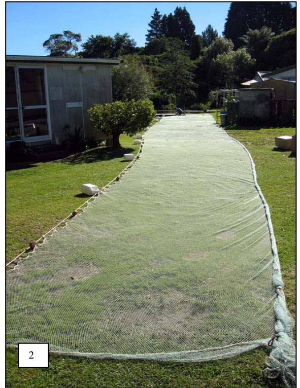
Plate 1. Enclosure net, showing the main net and the synthetic garden shade cloth end attachments.
