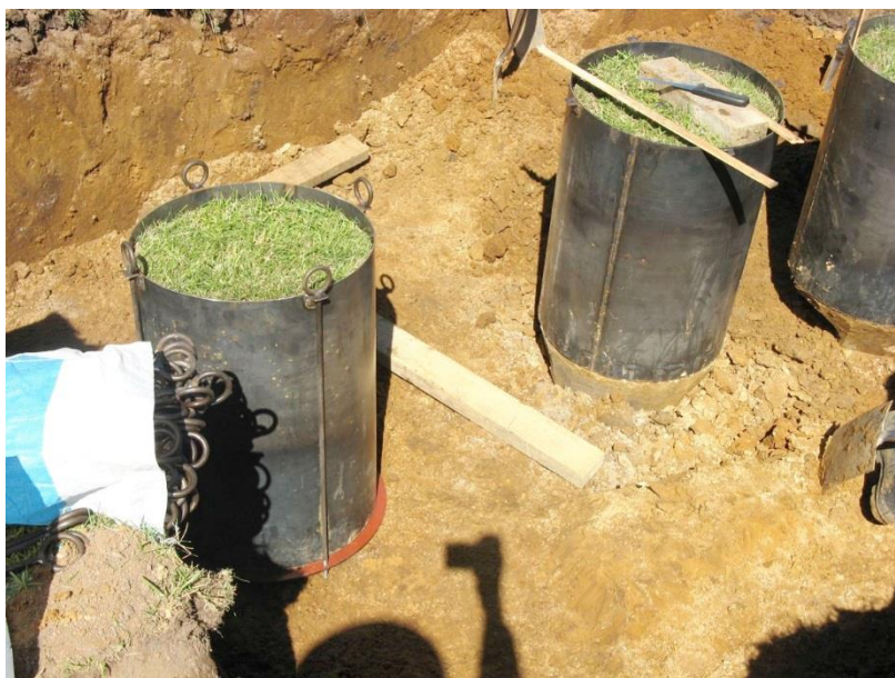
Figure 1. Lysimeter cores (intact soil) being collected at Paterson farm.
