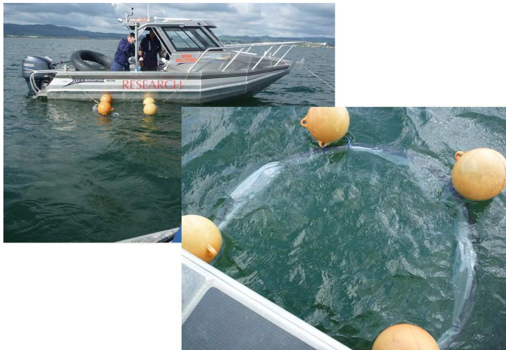
Figure 4: The 15 m deep settling chamber tube suspended from surface floats and tethered to the research vessel which used a 2-point mooring to hold position in the light breeze.
