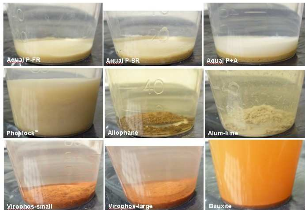
Figure 2: Products (2 g/100ml) as settled for 24 hours after 5 days of agitation and periodic vigorous shaking. Both bauxite samples remained highly turbid (only one shown).
