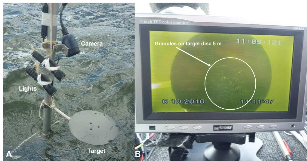
Figure 5: A) Drop-cam assembly showing the camera and black disc target plus the auxiliary lighting (xenon torches). B) The arrival of the product being tested on the target disc was very obvious and the degree of disaggregation was clearly visible. (Test product Aqual P FR at 5 m shown).
