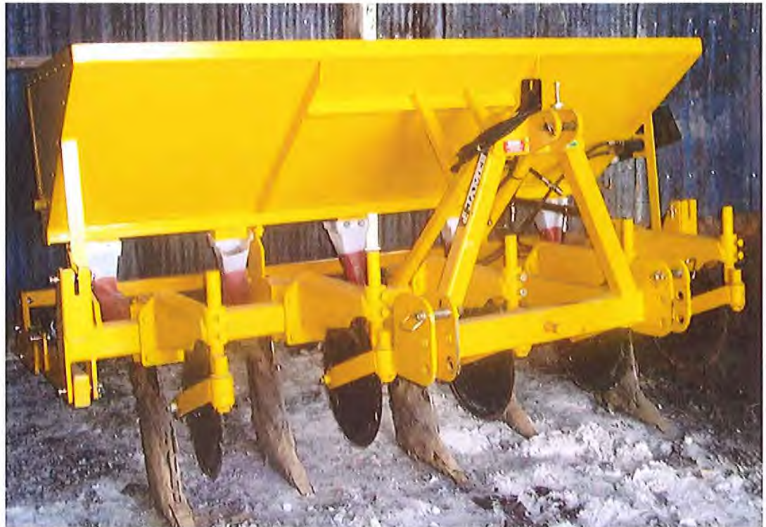
Modified James Engineering 5 tine subsoiler showing attached hopper and feeding tubes behind each tine
