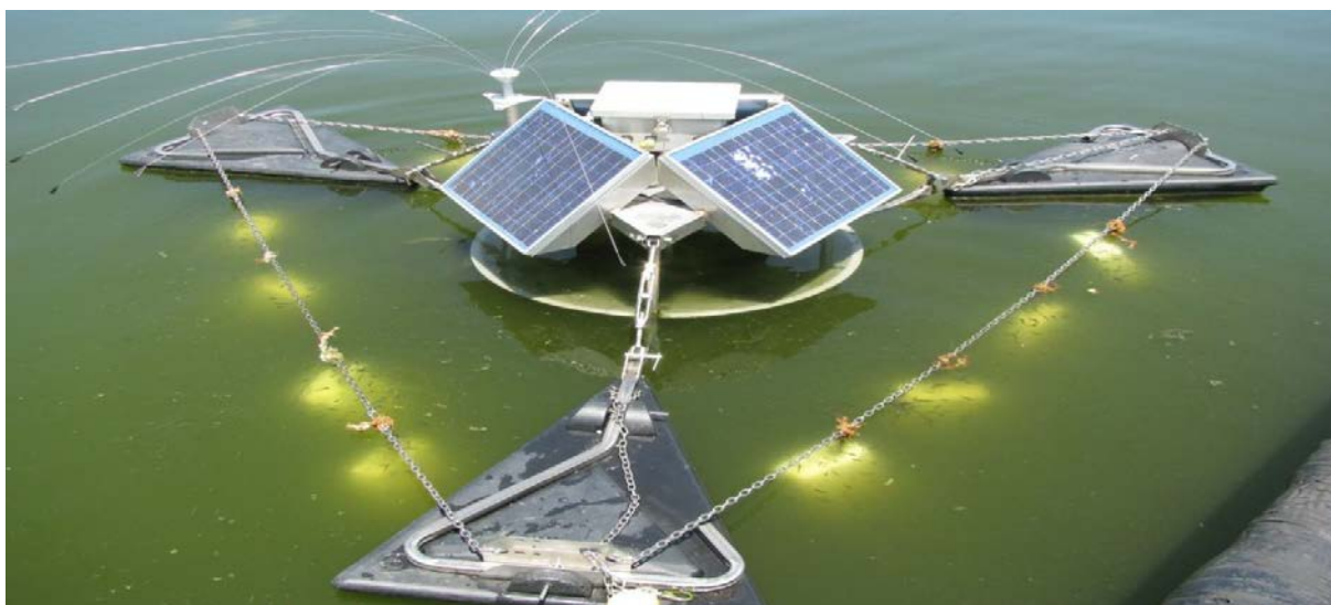
Figure 3: PAM slow release blocks secured in the outwards current flow from the SolarBee mixer.
