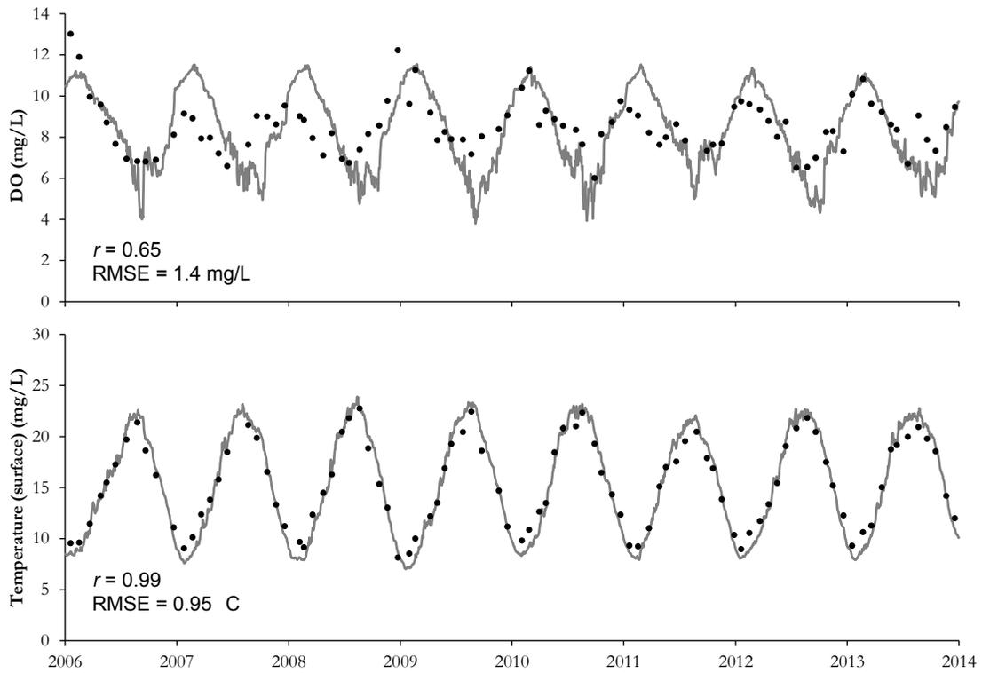
**Figure 17** Comparisons of measured (circles) and modelled (line) surface concentrations of dissolved oxygen (DO) and temperature.
