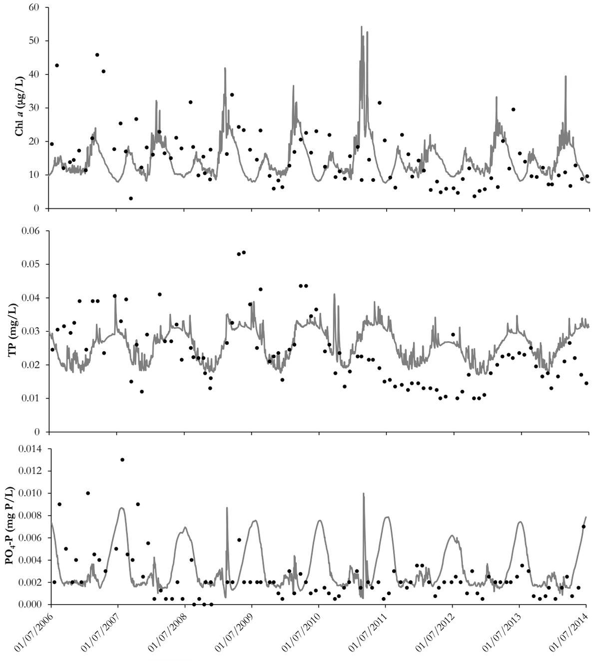
**Figure 19** Comparisons of measured (circles) and modelled (line) surface concentrations of chlorophyll *a* and phosphorus fractions. The detection limit for PO<sub>4</sub>-P was 0.008 mg P/L prior to October 2009, and 0.001 mg P/L thereafter.
