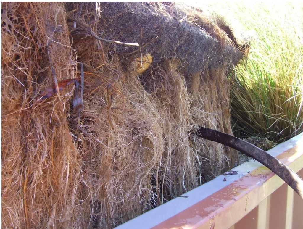
Figure 5: View of the extensive subsurface root development in the flow-through mesocosms by the end of the trial ( FTWs temporarily raised out of the water).
