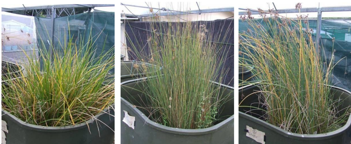
Figure 3: Batch-fed mesocosm tanks showing FTWs planted with Cyperus ustulatus , Juncus edgariae and Schoenoplectus tabernaemontani (left to right).
