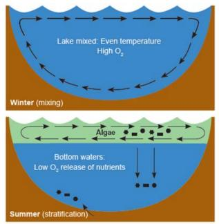
Figure 2 Diagram of lake dynamics during mixing and stratification
