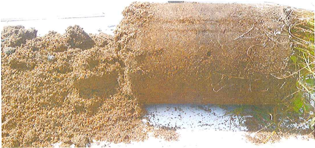
4) 45tonne/ha CNLZ – good penetration of roots down to drainage gravel
