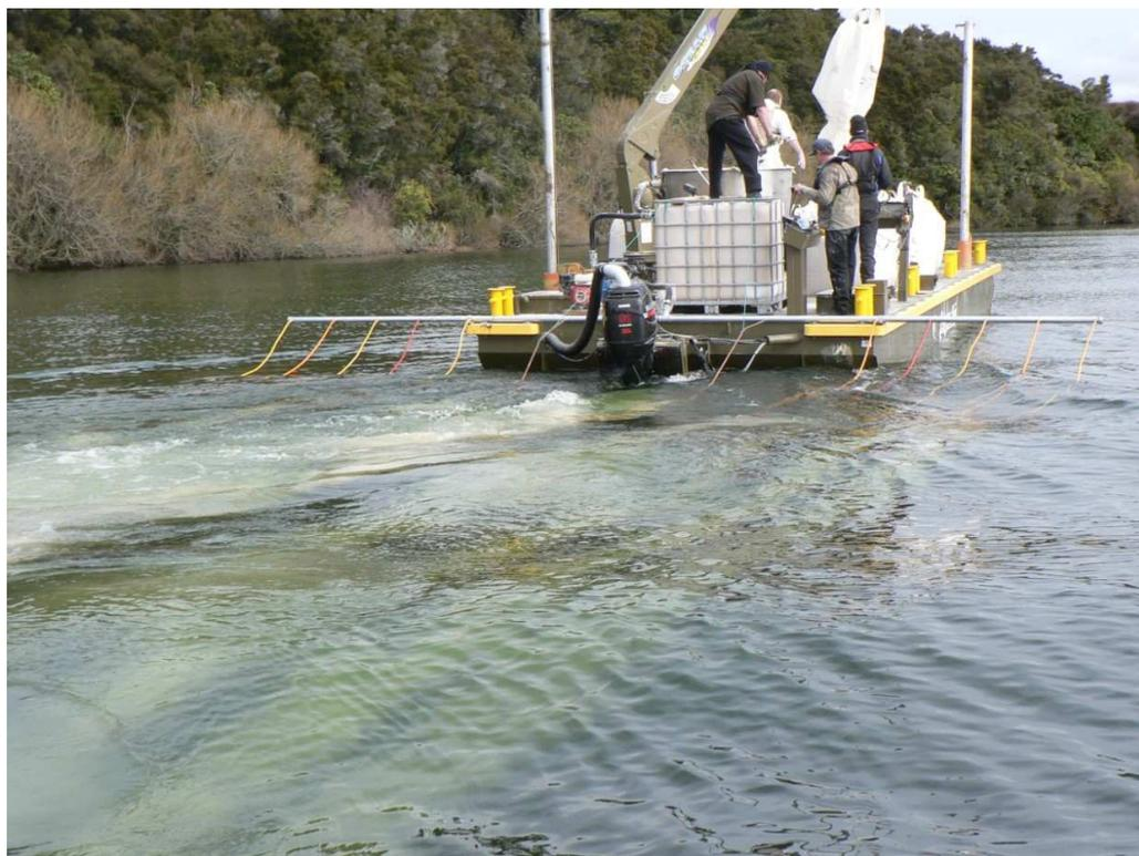
**Figure 3:** Application of the Z2G1 as a slurry, via spreader nozzles on the hoses from the boom across the back of the barge. The Z2G1 was mixed with lake water in the stainless steel mixing bowl at the back of the barge. The plumes of slurry can be seen deep in the water behind the barge. Photo by M. Gibbs. (See also cover photo).
