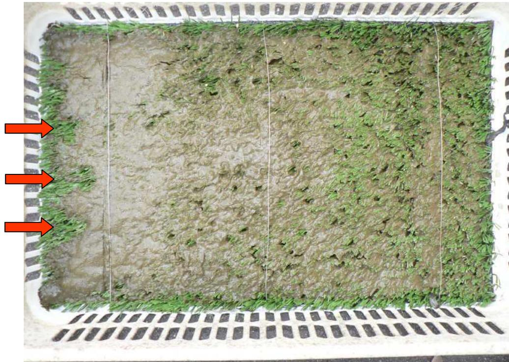
**Figure 4:** Sediment “Mat” trap uses 0.1 m<sup>2</sup> of artificial grass in a weighted flat tray placed on the lake bed to assess the evenness of the sediment coverage by the Z2G1 application. Trap from site 1 – the Z2G1 has settled between the artificial grass fibres but local variability in coverage also shows Z2G1 on top of the fibres. Three bully wallows can be seen on the left-hand edge of the mat (red arrows).
