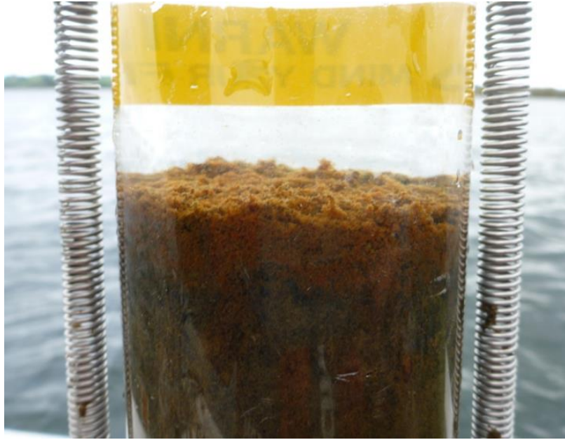
Figure 14 Iron floc on surface ~ 2cm thick, Lake Rerewhakaaitu (Photo credit; Max Gibbs, NIWA).
